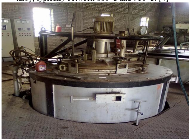
Figure 2.2 GAS CARBURIZING FURNACE
